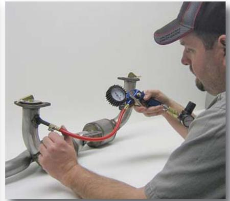
**All parts are pressure-checked before being shipped.**
