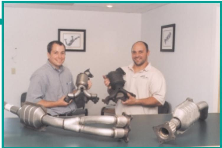
Ray Surprenant (left) holds a Davico direct-fit replacement converter and exhaust manifold for 1996-2000 Honda Civics, while Bob Hamel holds the OE unit. In the foreground are converters for 1999 and 2000 VW Jetta applications (left) and 1997 and 1998 Dodge Caravans.
