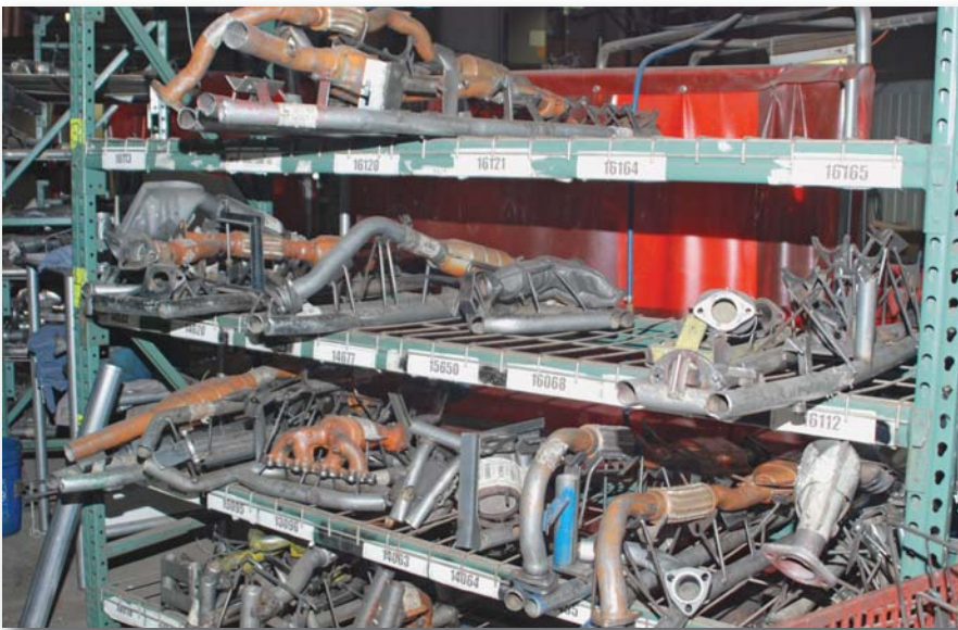
Fixtures for every part number are kept on hand to guarantee a perfect fit.
