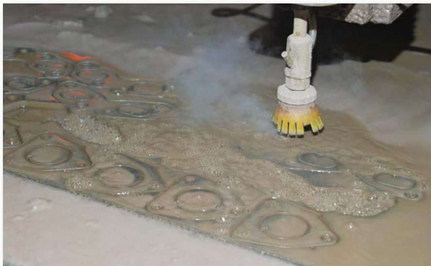
Davico uses a water-jet cutting machine for prototype and single-order flanges. It produces 50,000 pounds per square inch of pressure and eliminates distortion that a plasma cutter can cause. The unit also is used to cut flanges for motorcycle exhaust and to make surgical-tool handles.
