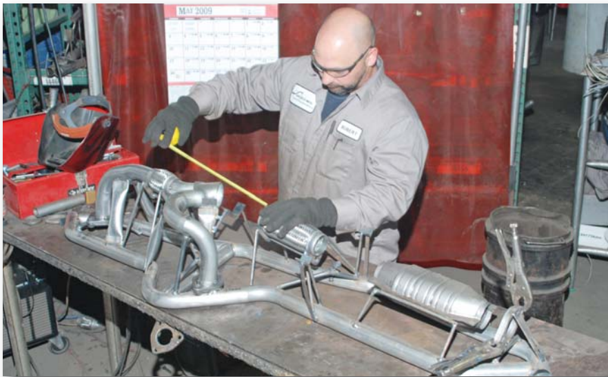
Robert Hamel, new-part development, builds a prototype converter system for a 2003 Mitsubishi Galant.
