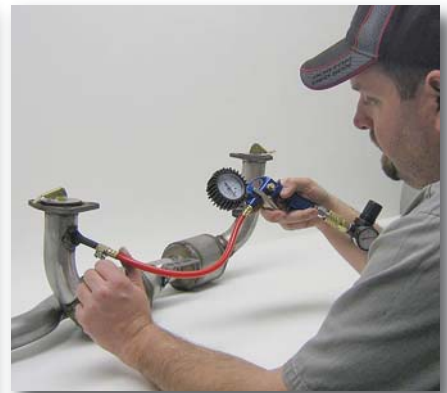
All parts are pressure-checked before being shipped.
